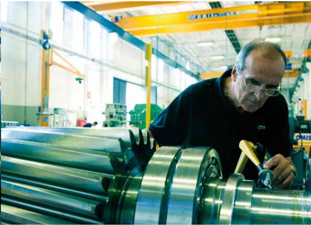
An inspector checks the precise roundness of a gear shaft.
