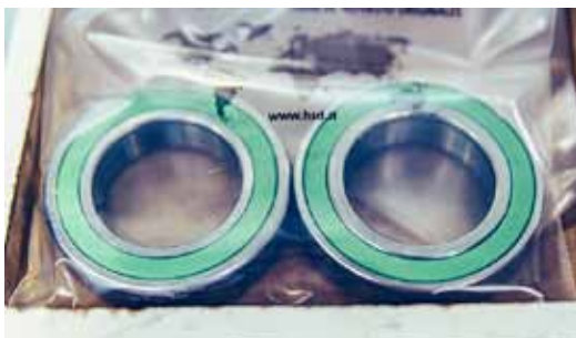
Above: Spindle shafts ready for balancing. Below: Bearings are kept in the original (sealed) packing until the very moment they are mounted.
