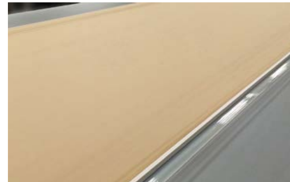
Below: Plasterboard is made by crushing gypsum and then adding water and additives. The mixture is transported along a long conveyor, called a forming belt.
